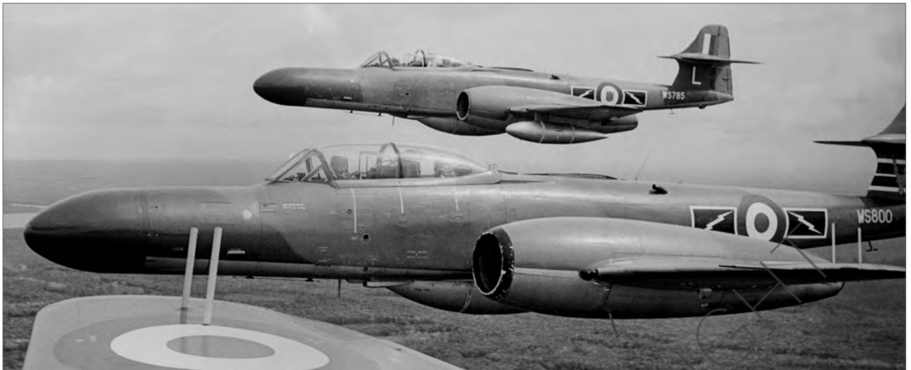
The Boss's aircraft, NF.14 WS800/A of 60 Sqn with striped fin, badge, and Sqn Ldr's pennant on the nose, and also the DME aerials above the outer wings. (D.W. 'Jok' Warne)
