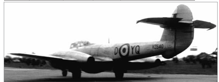
Meteor T.7 VZ640 YQ-D of 616 Sqn during the F.4 era, with early blade dorsal aerial.
